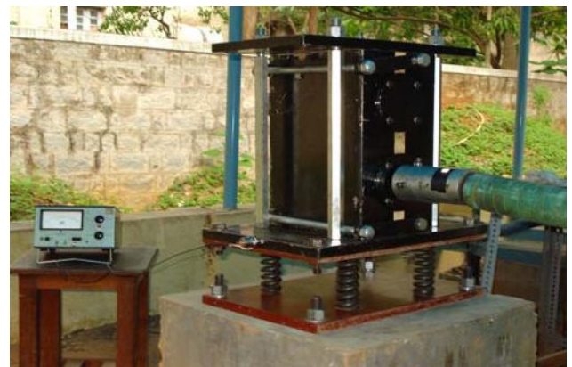
Figure: Model test setup for determining interference of two footings.
